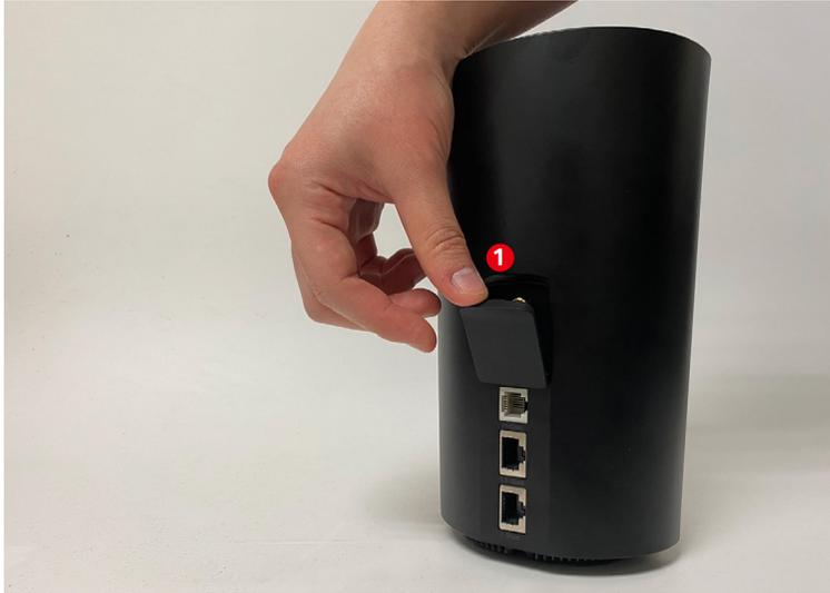
2. Connect your 5G external antennas to the antennas ports.
